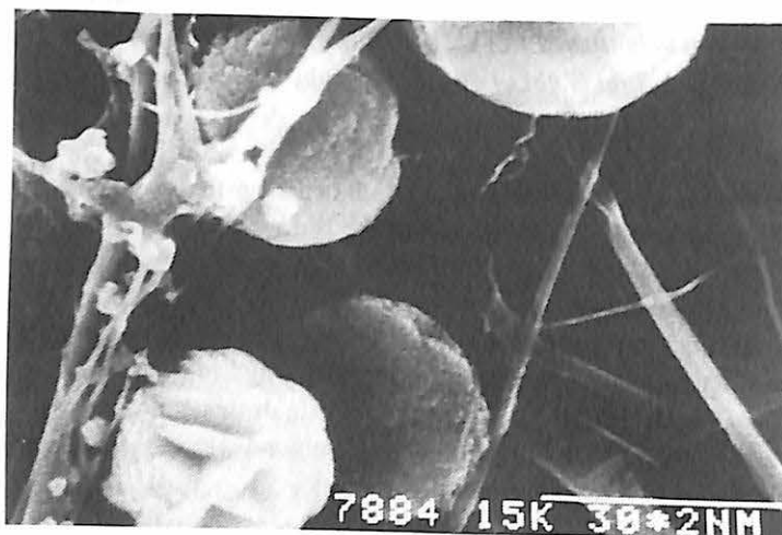
Figure 8. Celestite globules (those, where crystals are seen), silicate globules and threads from the foam, replacing gypsum gemmiforms from inside. SEM photo by A.Semikolennykh.
