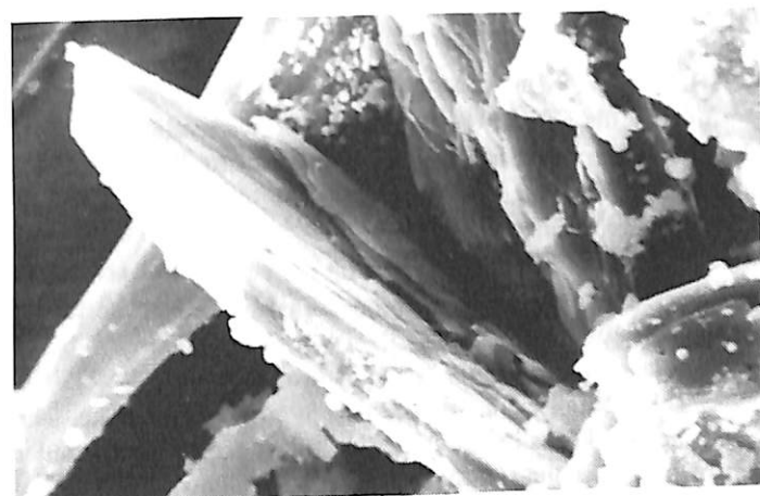
Figure 1. Gibbsite crystal in okher, 0.1 mm large, diagnosed via X-ray microzond. SEM photo by A.Semikolennykh.
